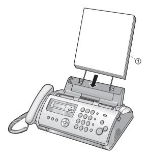
If the paper is not inserted correctly, remove all of the installed paper, and re-install it gently.
